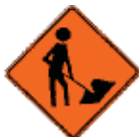
The Workers sign is used to alert drivers of workers in or near the roadway.
