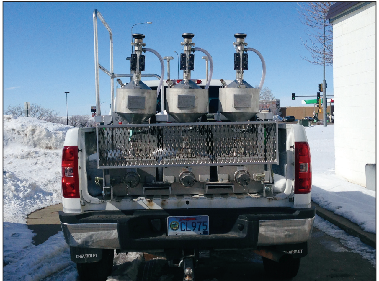
A new prover was purchase by Inspections/Weights & Measures in 2017. The prover, which can be placed into the back of a pickup, is a fuel test measuring device.
