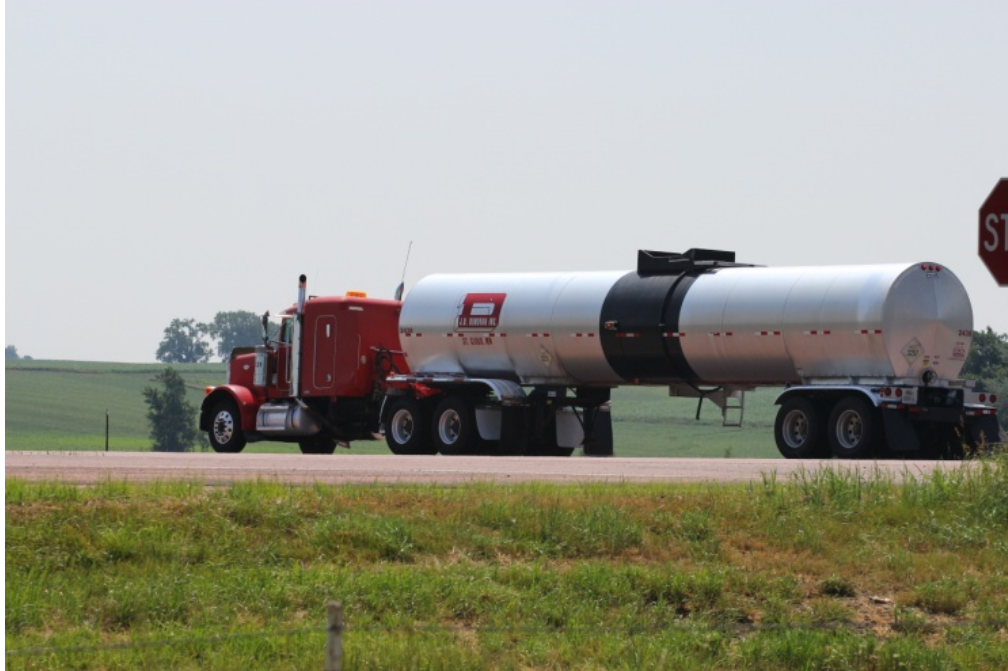
Figure 8 Class 9 – Elevated Temperature Liquid (UN 3257) in Low Pressure Chemical Tank
