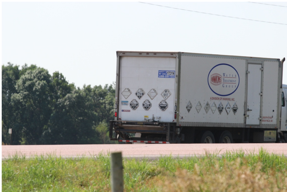
Figure 7 Division 2.3 – Chlorine (UN 1007) and Corrosive Materials in Mixed Cargo Vehicle
