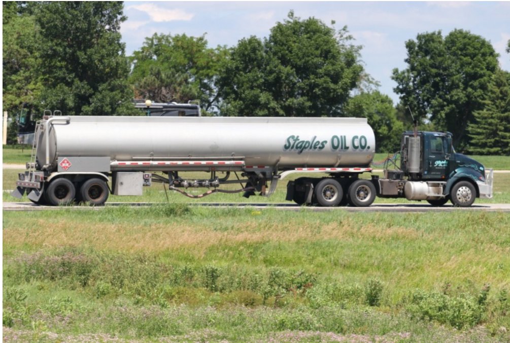
Figure 6 Class 3 – Gasoline (UN 1203) in Non-Pressure Liquid Tank
