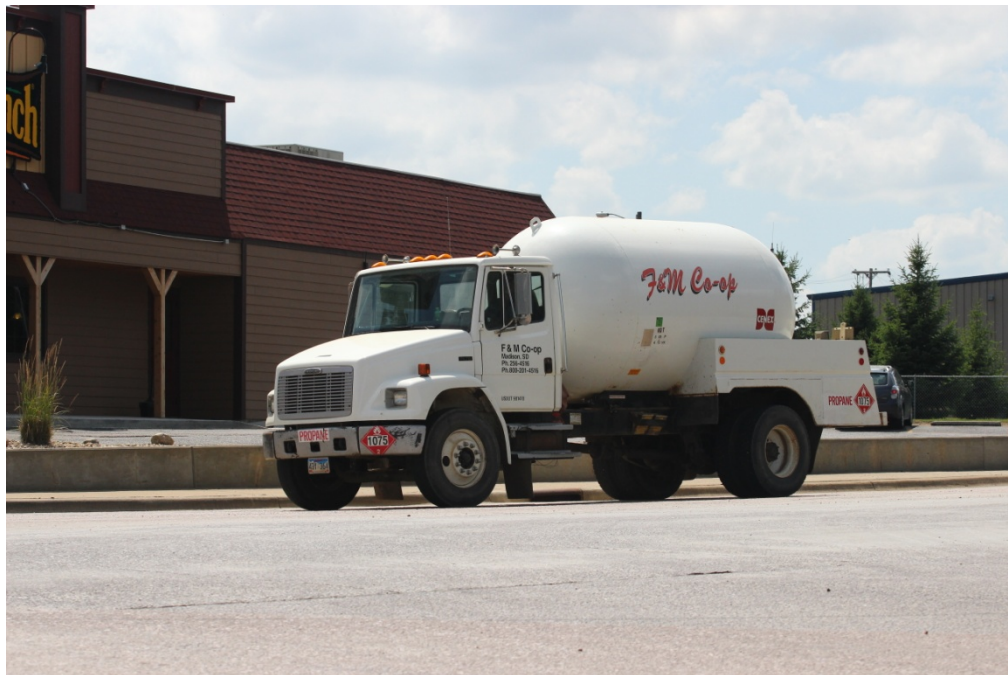
Figure 9 Division 2.1 – Propane (UN 1075) in High Pressure Tank
