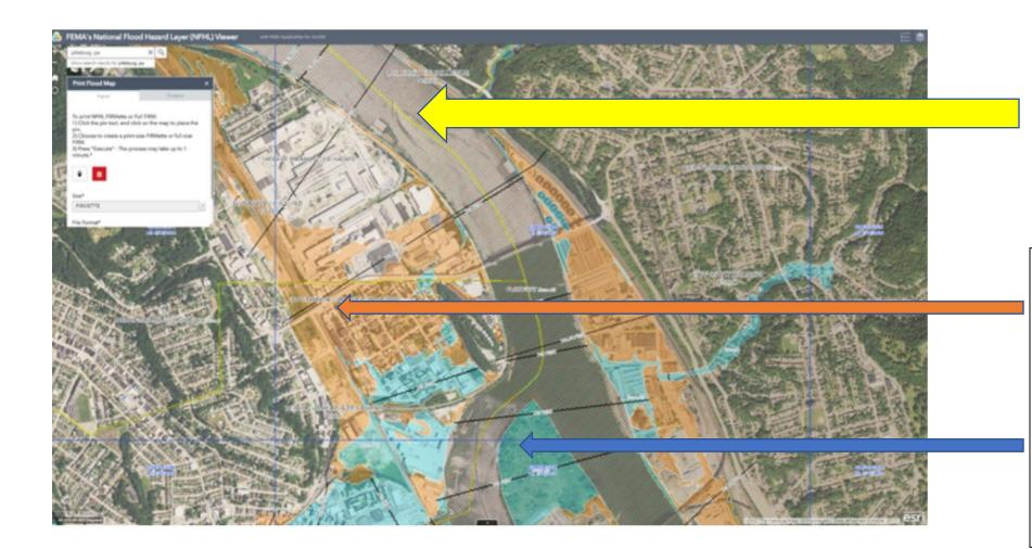
Regulatory Floodway. Channel of river. No action can be taken in the floodway that will increase water elevation. Permitting will be required for work in floodway. See your Local Floodplain Administrator
